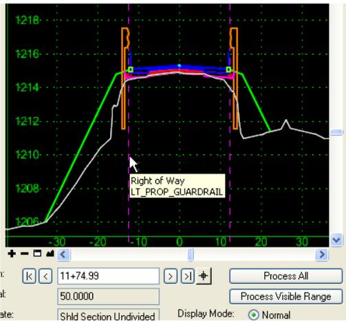
Note the priority of the guardrail graphics has recently been changed to override the guardrail fill height/slope warrant condition.
