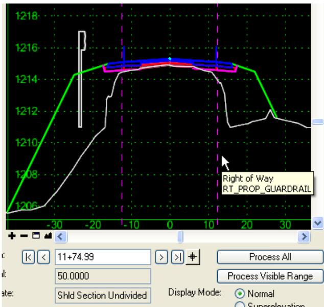
Not only is this normally not constructed, but the guardrail graphics are on the opposite side of the search range. Change the paved shoulder width to 0.01' (assuming no paved shoulder) and now the guardrail graphics are displayed in Roadway Designer.
